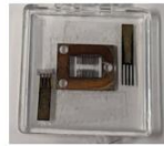
Figure 5.1: Connectors fabricated using a combination of desktop fabrication tools
