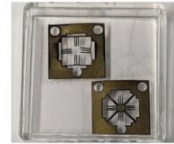
Figure 5.1: Connectors fabricated using a combination of desktop fabrication tools
